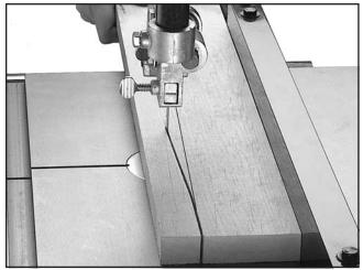
Figure 74. Example of blade lead.
